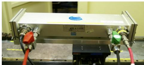
We measure the current produced by ionization of gas by incoming x-ray.
